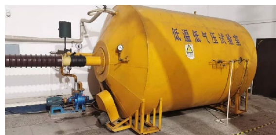
Fig. 4 Low temperature and low air pressure test chamber
