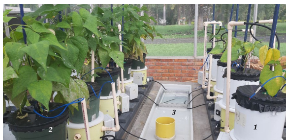
Fig. 6 Prototypes with plants—two groups. 1. Right—5 prototypes with younger plants (PCS) (1 month after sowing). 2. Left—5 prototypes with older (PCH) plants (> 80 days after sowing). 3. Center—water source container for prototypes' automatic daily irrigation supply
