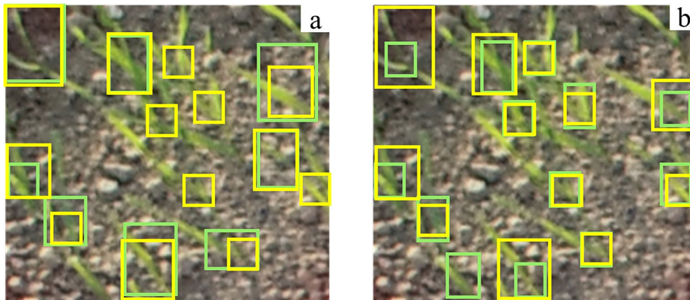
Fig. 9 Detection results of the model without the SPD-Conv module (a) and with the SPD-Conv module (b). Yellow boxes represent annotation, and green boxes represent detection
