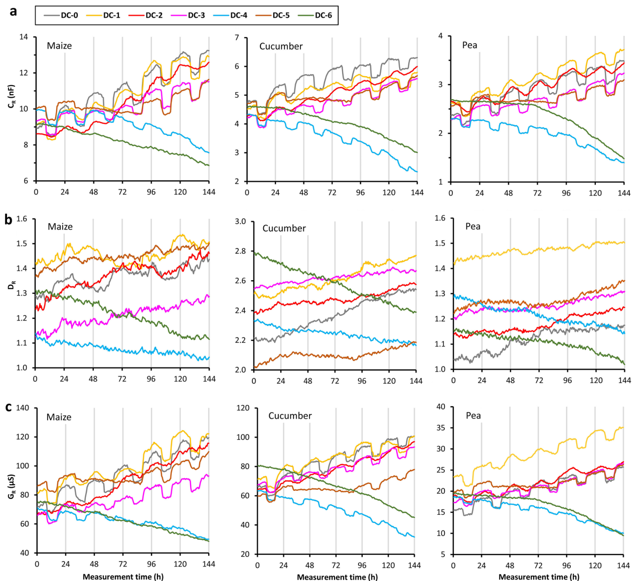
Fig. 3 Time series of a root electrical capacitance ( C_R ), b dissipation factor ( D_R ) and c electrical conductance ( G_R ) for maize, cucumber and pea in the diurnal changes (“DC”) experiment. See the text for the treatment codes
