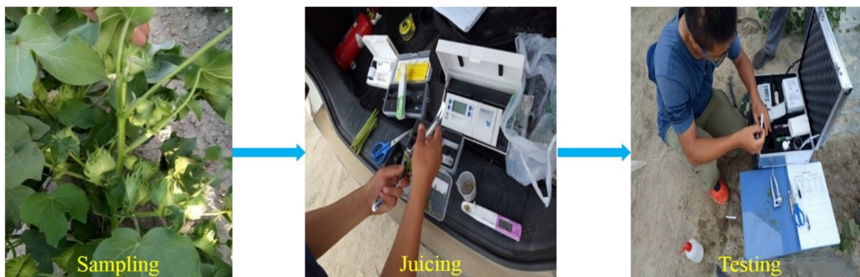
Fig. 2 Petioles NO 3 - -N, PO 4 3- -P and K + -K test procedure
