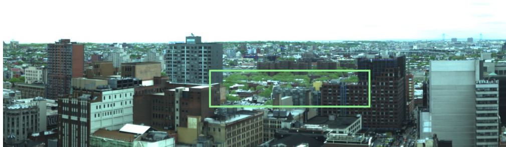
Fig. 2 A false-color RGB (0.61 \mu\text{m} , 0.54 \mu\text{m} , and 0.48 \mu\text{m} ) image of the scene of Downtown and North Brooklyn obtained by the Urban Observatory's hyperspectral imaging system. In the green box are the highlighted vegetation pixels relevant to this work, which are located at roughly 1 km south of the sensor that is sited atop a 120 m tall building
