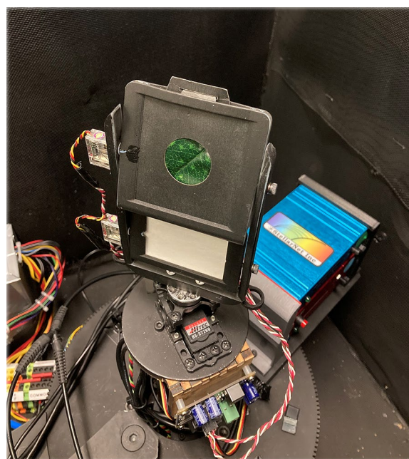
Fig. 1 Leaf holder used to ensure the same part of the leaf is assessed in every stage of the data collection
