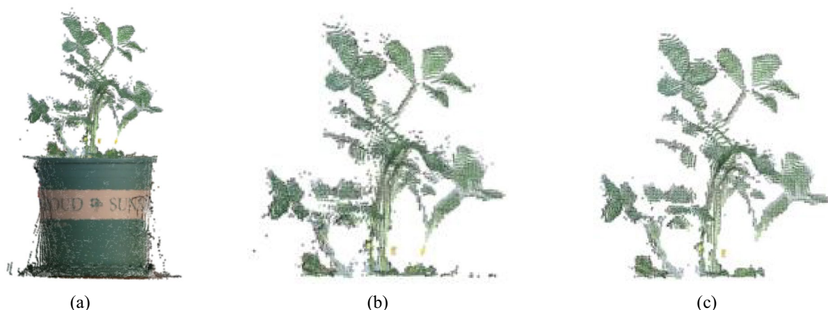
Fig. 5 Data filter results. a 3D color point cloud. b PassThrough filtering result. c Statistical filtering result
